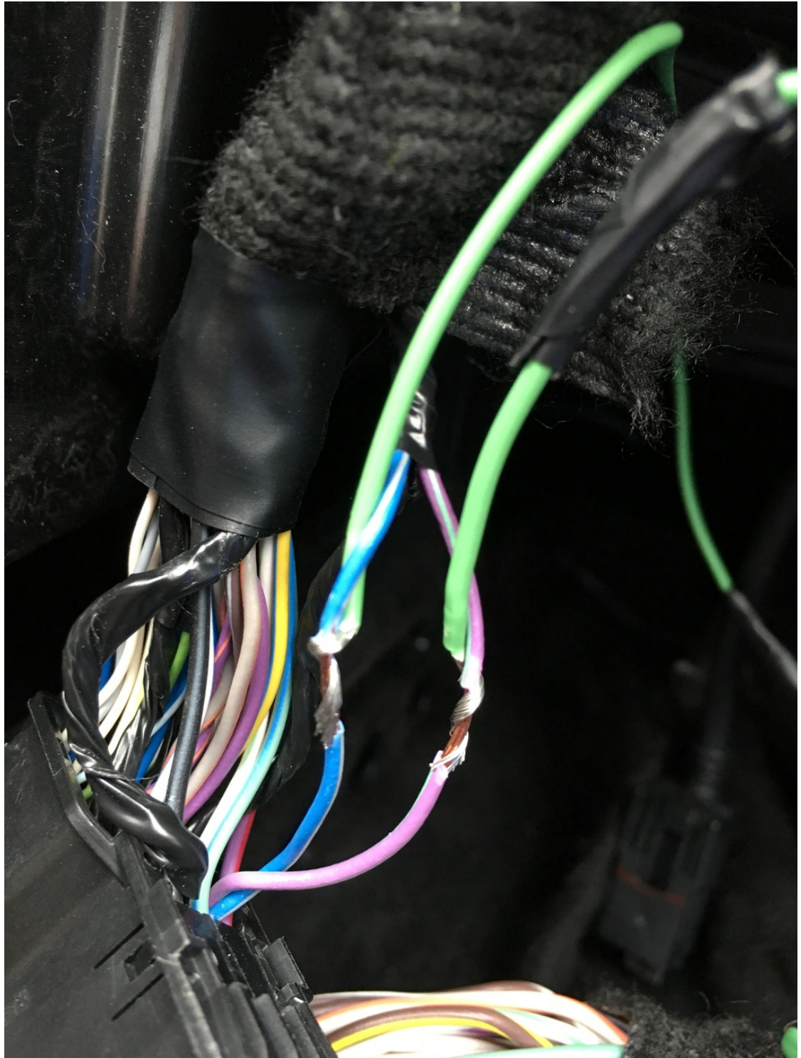
APIM Harness Wiring Taped Back Up:
