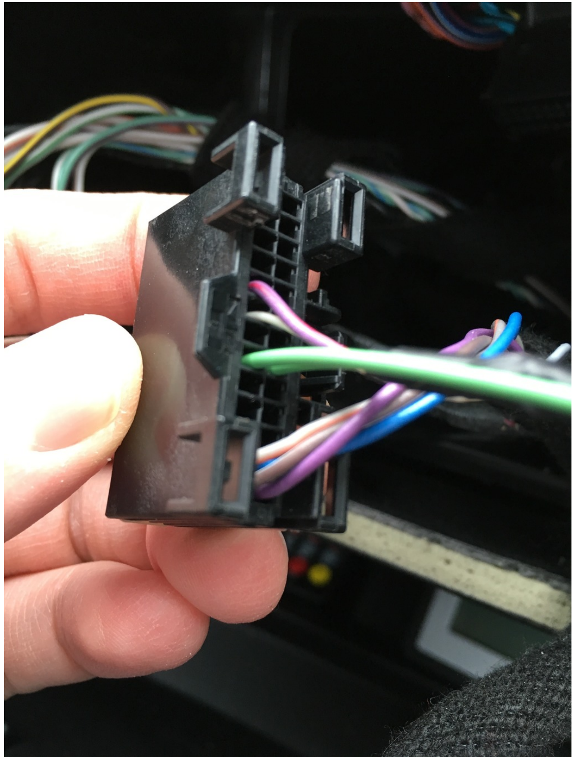
Other End of Wiring Terminal Connected to APIM Harness (Pins 3,4): ... MUST BE SOLDERED BEFORE TAPING WIRE UP...
